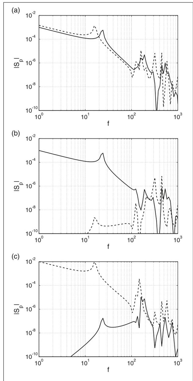
Figure 3. Numerical results for a manipulation of the source descriptor orders: (a) source with off-center force excitation; (b) source with force excitation at the center of mass; (c) source with off-center moment excitation. — zero-order source descriptor; - - - first-order source descriptor.
