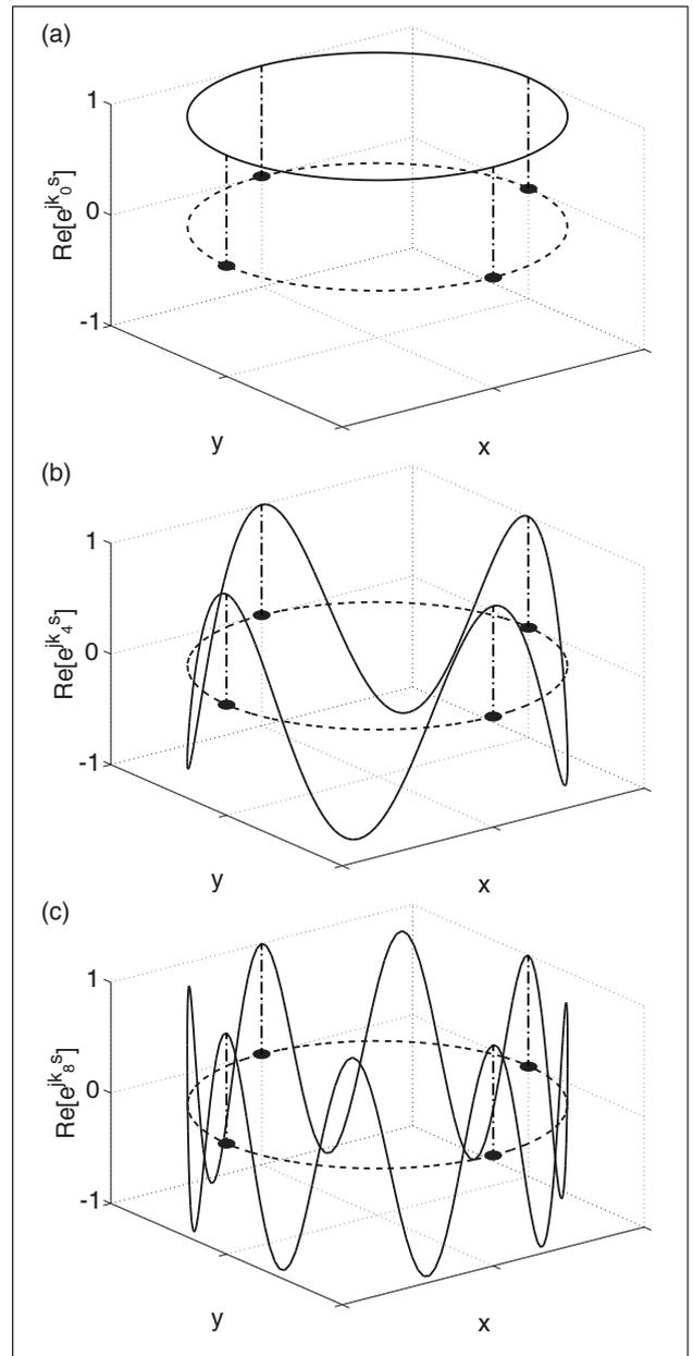
Figure 2. Illustration of the order decomposition for a continuous velocity distribution along a circular contour: (a) zero order; (b) fourth order; (c) eighth order. — order distribution; - - - contour; - · - · - amplitude at sampling point; • sampling point.
