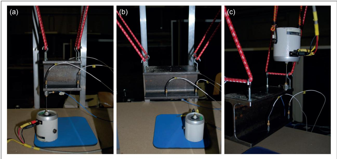
Figure 4. Experimental setup for measurements on laboratory source structures: (a) mobility measurement; (b) mobility measurement on enlarged source; (c) free-velocity measurement.
