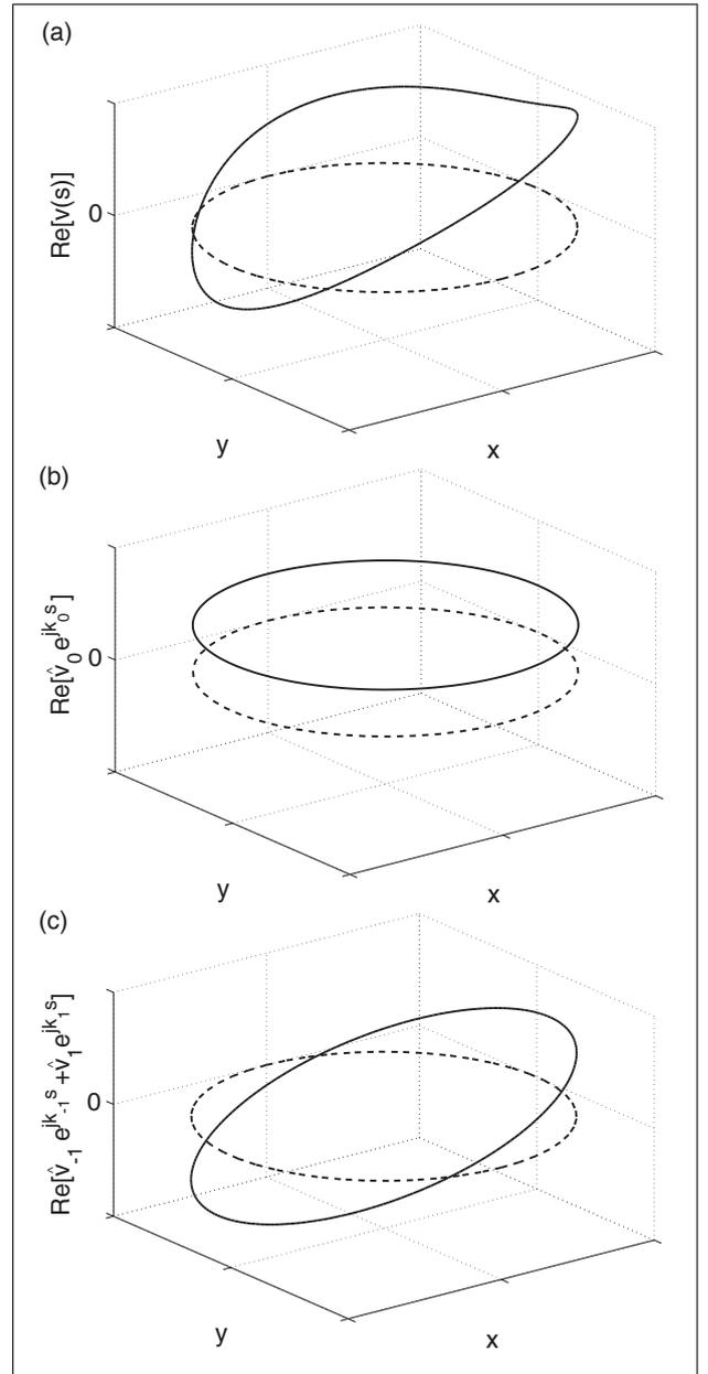
Figure 1. Illustration of the order decomposition for a continuous velocity distribution along a circular contour: (a) spatial velocity; (b) zero-order velocity; (c) first-order velocity. — velocity; - - - contour.
