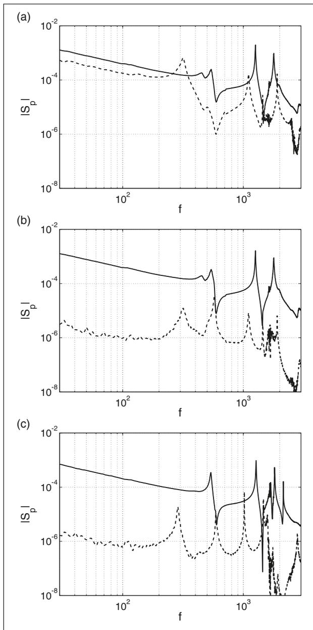
Figure 5. Experimental results for a manipulation of the first-order source descriptor: (a) source with off-center force excitation; (b) source with force excitation at the center of mass; (c) source with attached structure. — zero-order source descriptor; --- first-order source descriptor.
